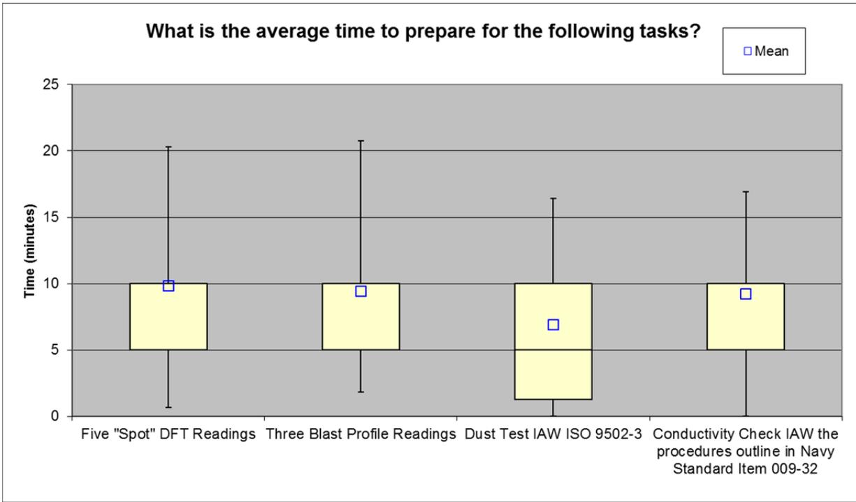
**Figure 2. Time required preparing for various coating inspection tasks during shipbuilding and repair.**
