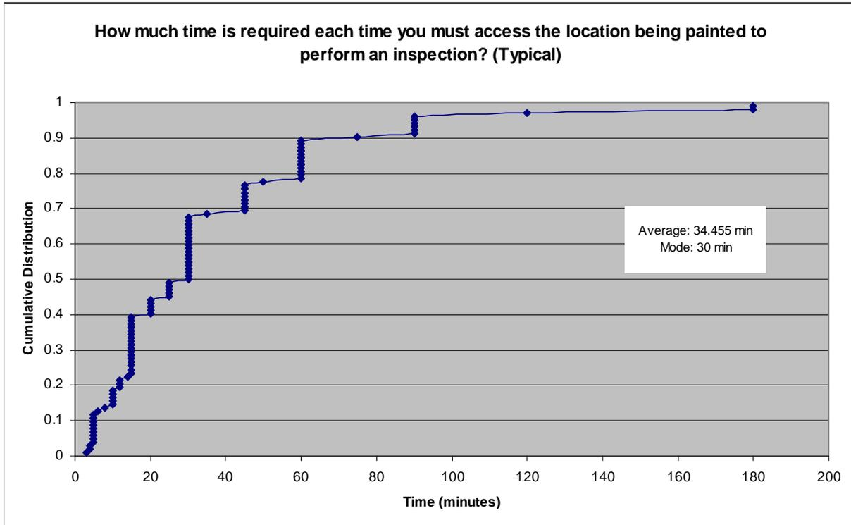
**Figure 1. Distribution of time required for an inspector to get from their work location to the surface being inspected during shipbuilding and repair.**
