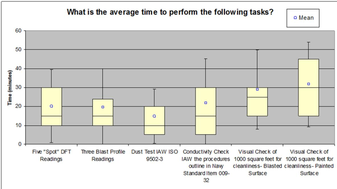
**Figure 3. Time required to perform various coating inspection tasks during shipbuilding and repair.**
