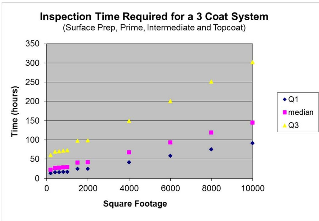
Figure 4. Model projections of the time required to perform coating inspections on various sized surfaces during shipbuilding and repair.
