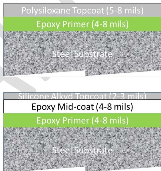
Figure 4. Legacy Navy 3-coat system (bottom) and new 2-coat Polysiloxane system (top).
