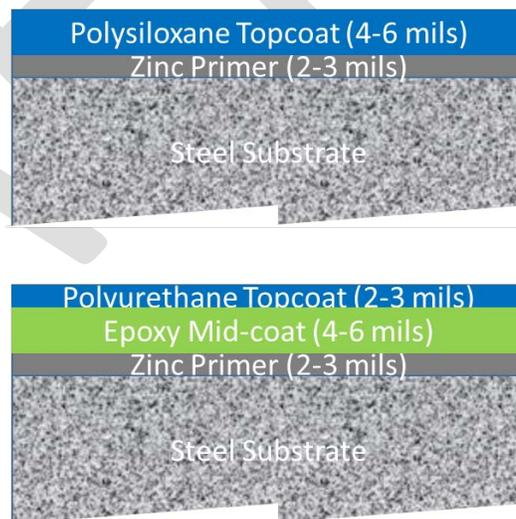
Figure 3. Typical 2-coat Polysiloxane system (top) and 3-coat Polyurethane system (bottom).
