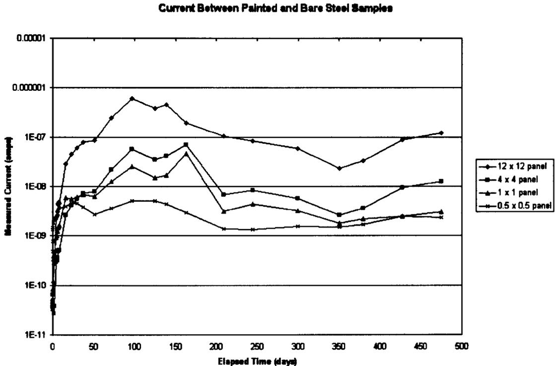
**FIGURE 1 - Average Current Between Exposed and Coated Steel.**
