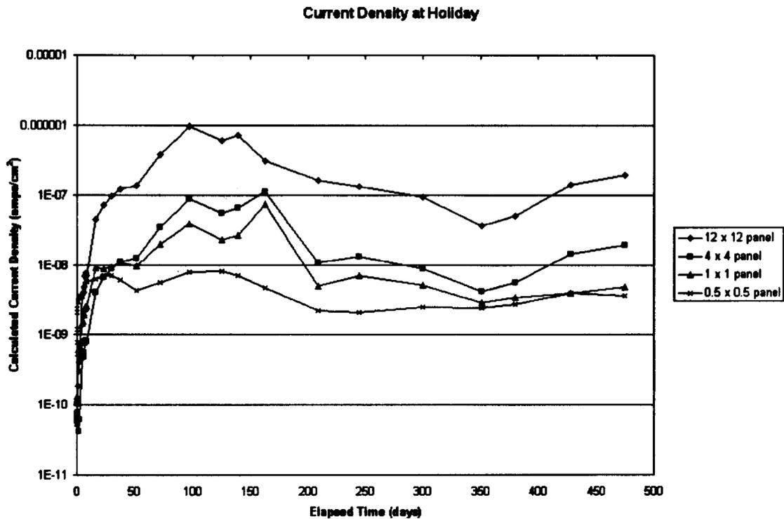
**FIGURE 2 - Calculated Average Current Densities at Coating Holidays.**
