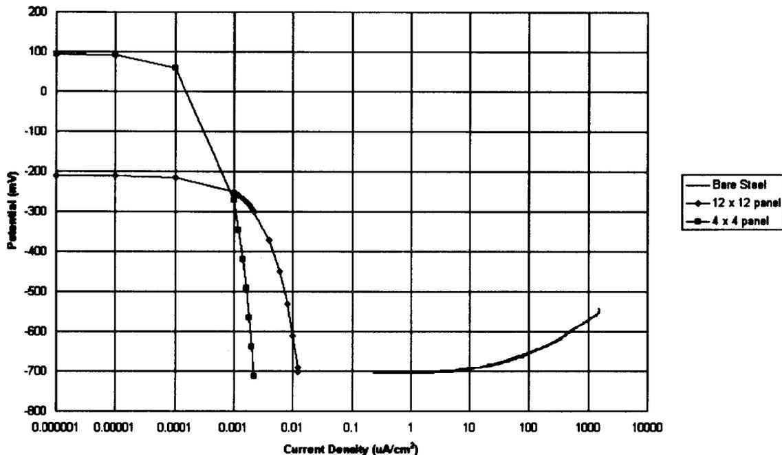
**FIGURE 3 - Polarization Scans of Bare and Coated Steel.**
